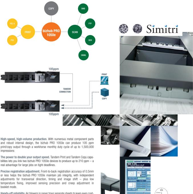
**Hands-off reliability.** Air blowers in paper trays separate sheets to keep even coated paper stock moving smoothly – and ultrasonic sensors detect misfeeds to prevent paper jams before they occur and maximize print production efficiency.
